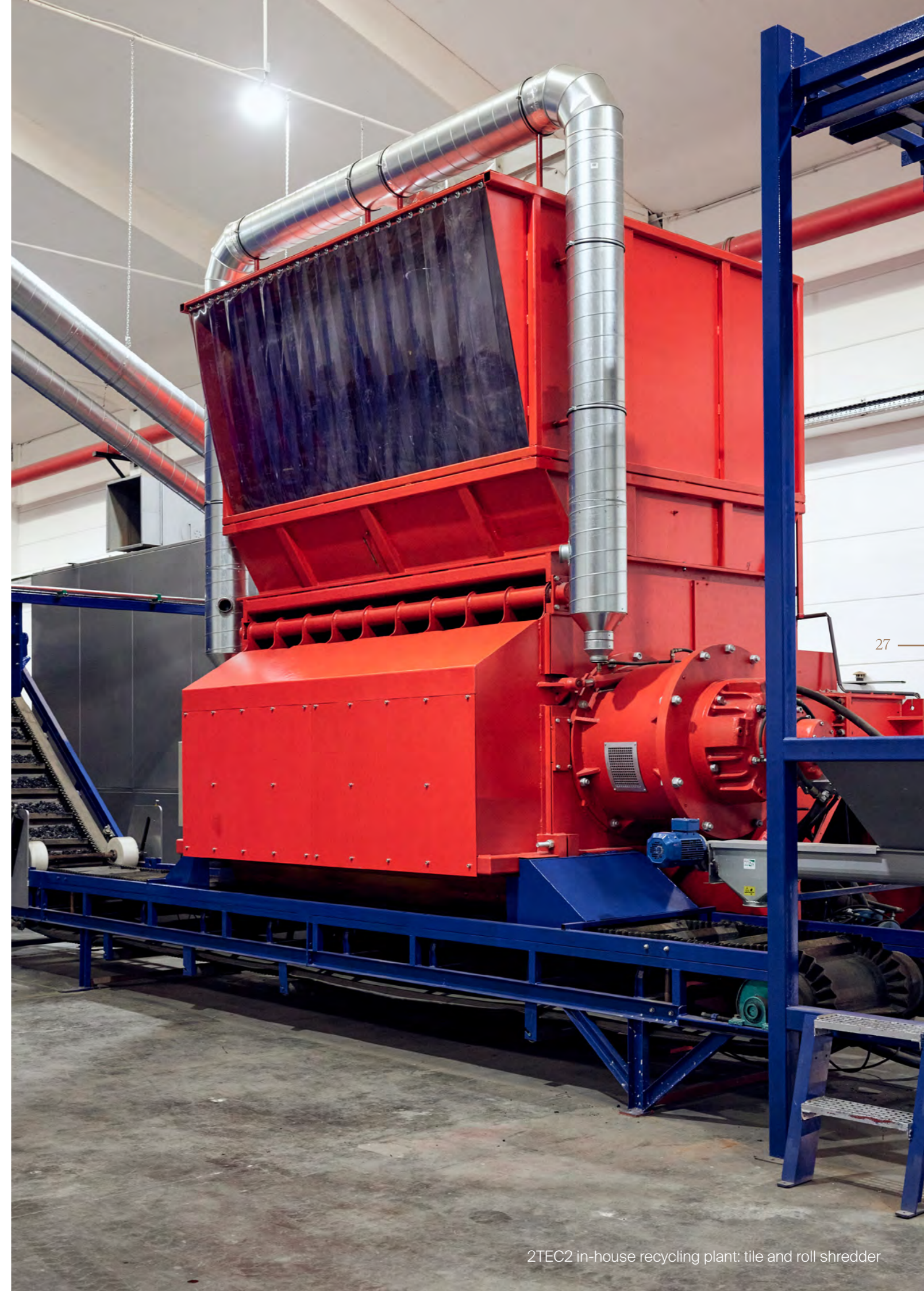
2TEC2 waste being shredded into new raw material
